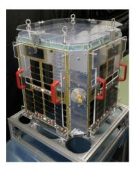
Nano-JASMINE, 5cm aperture, 35kg, 0.6 to 1.0 micron. Launch during Dec 2014 – Dec 2015
